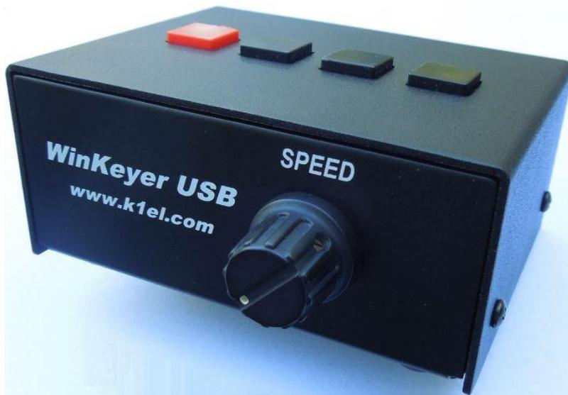
WKUSB, with a WinKeyer IC, is K1EL's original CW interface for the PC. It provides a convenient way to connect your PC to an amateur radio transceiver and send Morse both under computer control and by iambic paddle. Morse keying that is generated by a PC based application is prone to timing problems that are a result of the multitasking nature of Windows and other operating
